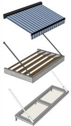
Retractable fabric, wood louver, or glass/metal sunshade canopies
